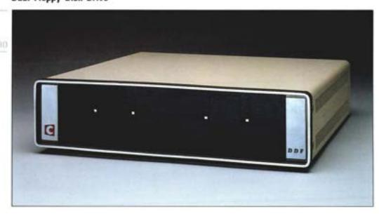
The Model DDF is a dual disk drive which is designed for use with Cromemco's System Zero. The double-sided, double-density drives provide a total of 780K bytes of storage.
