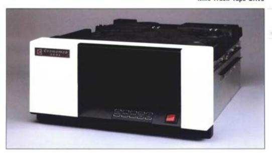
The Model TDS is a nine-track tape drive which provides large storage capability as well as data exchange with other IBM/ANSI systems using the 1600 bpi format. The drive can store over 40 million bytes on a reel of tape.
