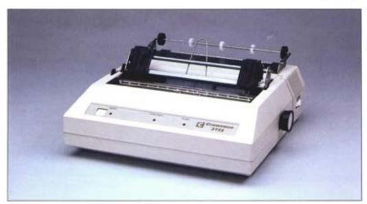
The Model 3715 is a dot-matrix impact printer that operates at 150 characters per second. Up to 80 characters per line can be printed at 10 cpi and up to 132 characters per line can be printed at 16.36 cpi. The unit prints 9 x 7 dot-matrix characters.
