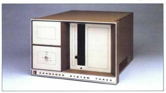
The basic System Three comes with a Z-80A processor, 64Kb of RAM memory, two 8" floppy disk drives which provide a total of 2.4 megabytes of storage, a 21-slot shielded motherboard, a heavy duty power supply, 110- or 220-volt operation, an all-metal chassis, and rack or optional bench cabinet mounting.
