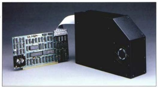
The Model HD-20 is a 21-megabyte hard disk subsystem which allows users who require large storage capacity to upgrade their systems. The Model HD-20 consists of a state-of-the-art Winchester technology disk drive and Cromemco's WDI-II hard disk interface card.
