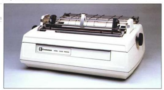
The Model 3355B operates at 55 characters per second with both tractor feed and friction platen for letter quality printing. The 3355B uses a reinforced plastic print element called a "thimble" that contains up to 128 fully-formed characters of various typefaces.
