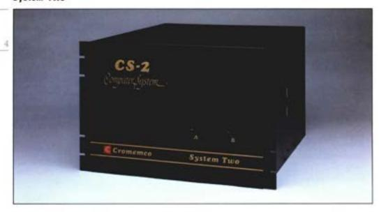
Cromemco's D-Series System Two is a rugged, industrial-grade, rack-mount computer that was especially designed for applications in areas such as industrial automation and process control. The System Two can also easily be configured for specific applications with Cromemco's add-on memory and I/O boards, including multi-processing, analog-to-digital, networking interfaces, and a variety of serial and parallel interfaces.
